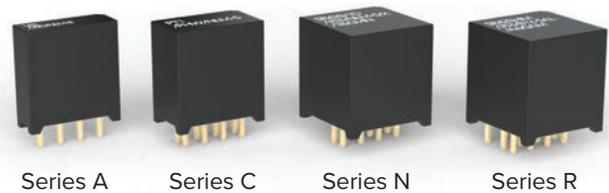
Part numbers are laser marked on the top of each component for easy identification after installation. Solderable pins (0.025" diameter) are designed to be compatible with 0.062" to 0.093" thick circuit boards.
