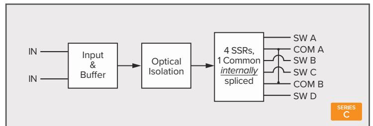
**Dual Switch Pair:** Four (4) SPST contacts (or switches) in two pairs connected with one common per pair.
