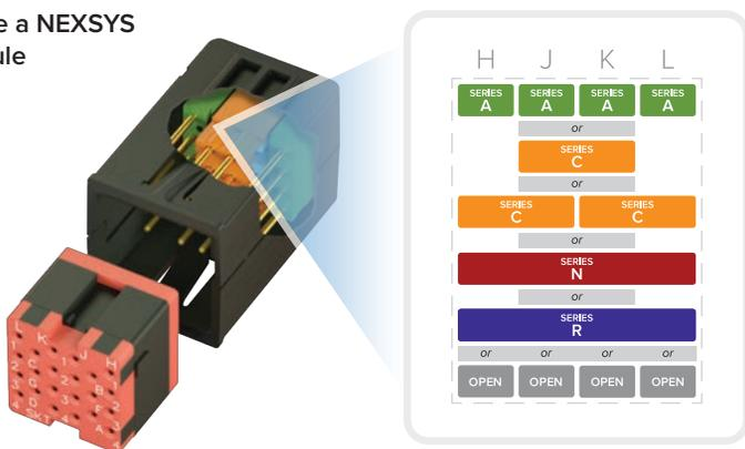
NEXSYS Modules have four available positions (H, J, K, and L in the diagram above). Modules can contain (a) up to four Series A components; (b) a single Series C component with up to two Series A Components; (c) two Series C components; or (d) a single Series N or Series R component. **See page 12.**
