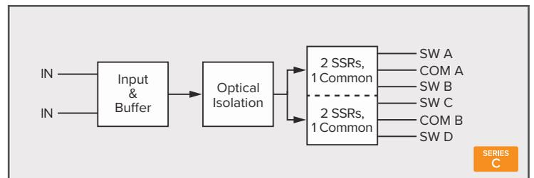
**Three Switch Single Common, One Switch Single Common:** Three (3) SPST contacts (or switches) connected to one common and one (1) SPST contacts (or switches) connected to another common.
