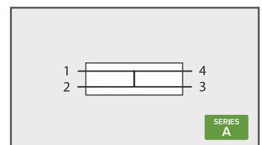
The Terminal Block (TB4) is rated at 5.0 A (max.) or 1.0 A (max.) when combined with an ARINC 429 Signal Converter, and provides an ability to bus a single input to three outputs.
